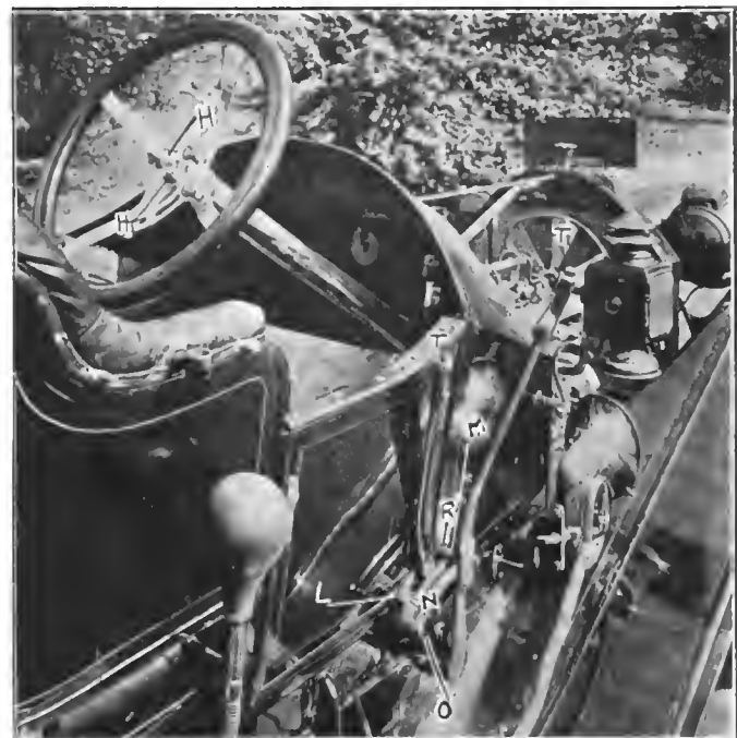
Fig. 6—Control levers on steering for ignition and throttle gear and brake
